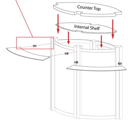
WHEN DISASSEMBLING ALUMINUM EXTRUSION, TIGHTEN ALL SETSCREWS AND LOCKS TO PREVENT LOSS DURING SHIPPING 866.652.2100
